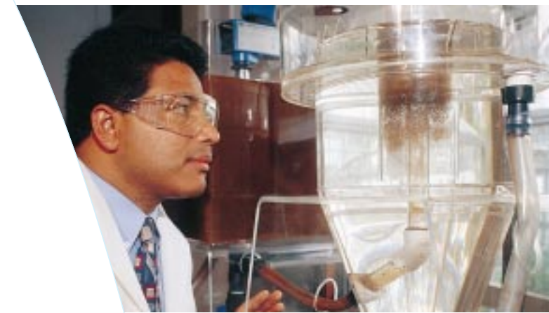
Ismael Sosa-Sanchez tests Orica's novel MIEX technology, which removes organic material from water to give it a clean taste, appearance and smell.
