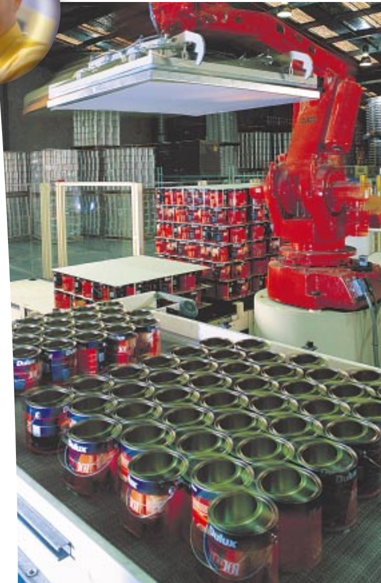
A robot loads empty paint cans at the start of the filling line at Rocklea (Queensland, Australia)
